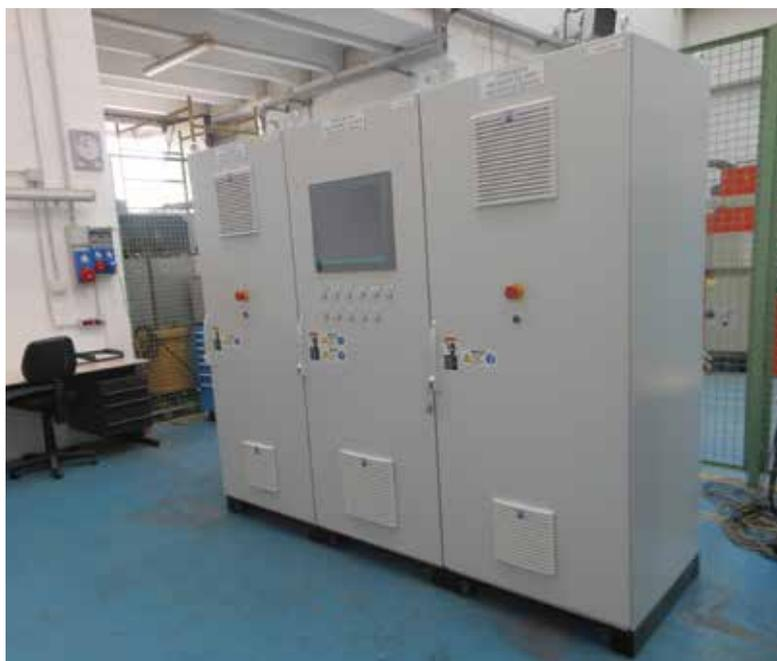
panel PC as HMI, manage the entire system through a redundant Siemens S7-400 PLC (Hot backup) and interfaces with the client's DCS by serial link. Furthermore, the PLC controls a package that is fully automatic and also implements all interlocks necessary to protect the plant and the personnel against operating faults or plant failures.
